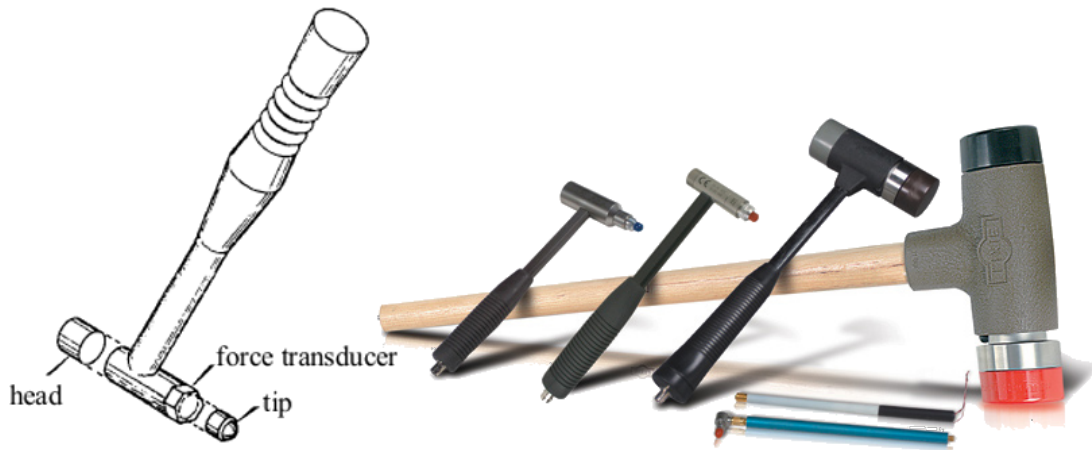
Figure 3.7. Scheme and examples of impact hammers [12, 1].
