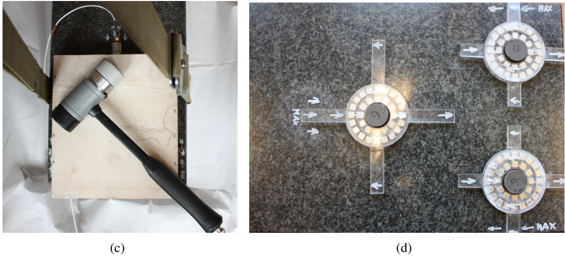
Figure 5.20. Pictures of the test stand: a) the whole test stand from the side, where visible are: upper and bottom plates, elastic bands and transducer; b) test stand from the front, where visible are: Hallbach arrays and both plates; c) picture presenting test stand from top with the impact hammer at the top; d) test stand without upper plate where three Hallbach arrays are visible with the MRE samples in-between.
