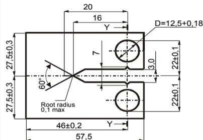
Fig. 7. CC(T) specimen (compatible with ASTM E 399-81)
