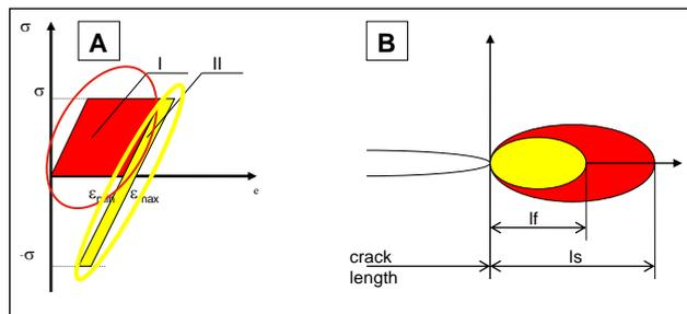
Fig. 5. Simple scheme of: a) external loading, b) plastic area ahead of a crack tip
