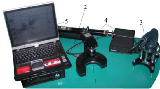
1 - speckle-interferometer; 2 - fiber; 3 - drilling device; 4 - laser; 5 - notebook
