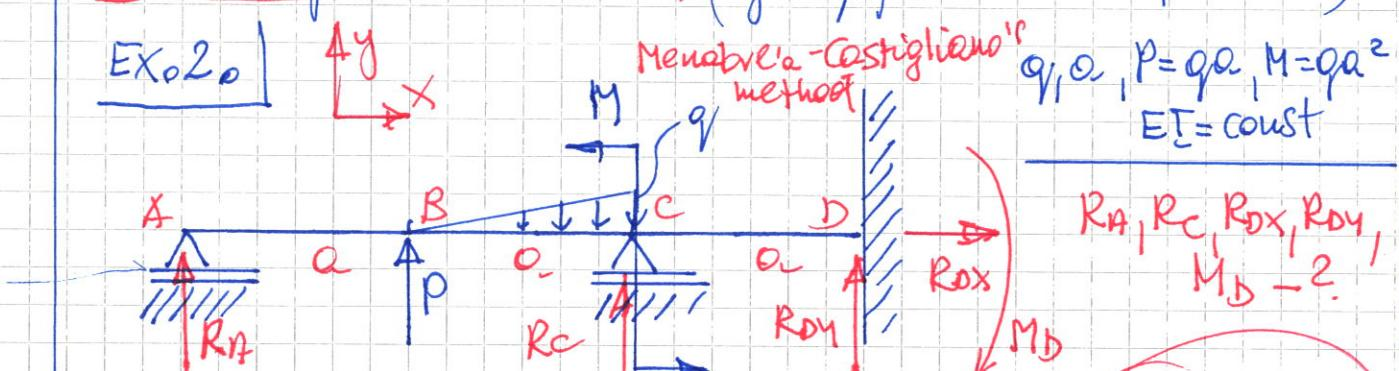
5 reactions - 3 static equations  $\Rightarrow$  2x hyperstatic beam
