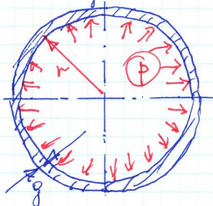
The pressure  $p$  acts on the cut-off part of the vessel, giving the force  $P$ , where
