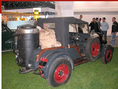
Gasifier is visible in the rear, the fuel storage on the roof. Along the roof and pillars, hot wood gas runs to the cooler mounted in the front of the vehicle.
