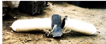
b) Vessel rupture
