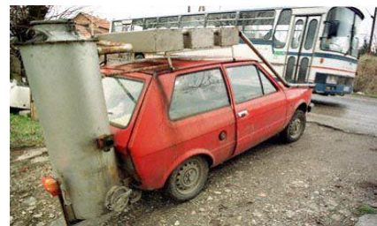
Gasifier is visible in the rear, the fuel storage on the roof. Along the roof and pillars, hot wood gas runs to the cooler mounted in the front of the vehicle.
