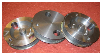
NOL specimens (photo and FEM model) as well as innovative displacement sensor heads
