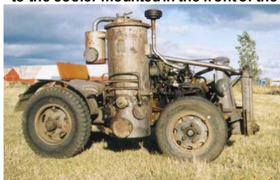
Gasifier is visible in the rear, the fuel storage on the roof. Along the roof and pillars, hot wood gas runs to the cooler mounted in the front of the vehicle.
