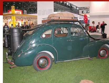
Gasifier is visible in the rear, the fuel storage on the roof. Along the roof and pillars, hot wood gas runs to the cooler mounted in the front of the vehicle.
