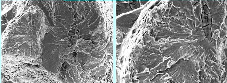
These round areas with transgranular cleavage mechanism on the background a ductile dimple structure of fracture surface were not founded in non-operational metal. Therefore, they were considered as fractography evidences of the degradation of metal from different zones of weld joint.
