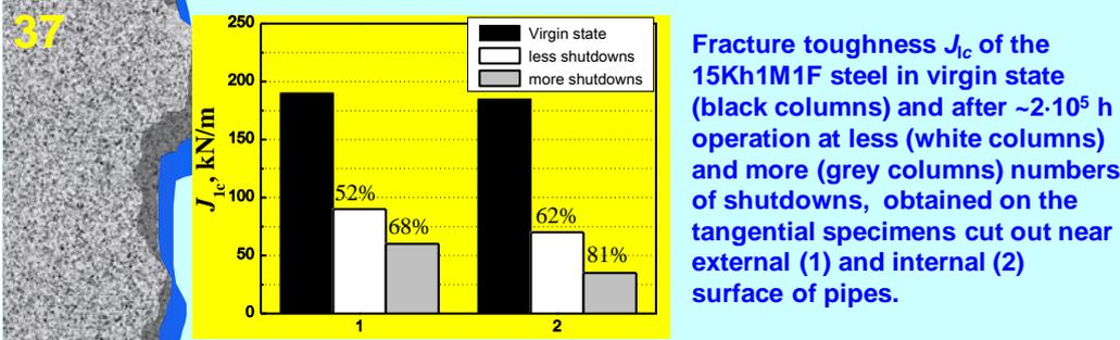
Fracture toughness  $J_{Ic}$  of the 15Kh1M1F steel in virgin state (black columns) and after ~2·10<sup>5</sup> h operation at less (white columns) and more (grey columns) numbers of shutdowns, obtained on the tangential specimens cut out near external (1) and internal (2) surface of pipes.
