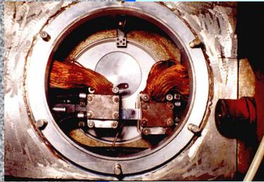
The method is based on the thermocycling of specimens in the hydrogen environment. The choice of temperature range is based on the information about the operating temperature of oil hydrocracking reactor or steam pipeline on the power plant.
