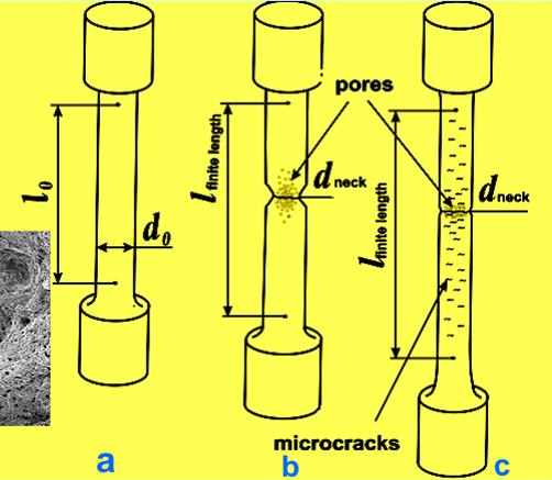
The scheme of specimens before (a) and after (b, c) tensile test in order to explain the abnormal change of the plasticity characteristics of the metal in the virgin state (b) and after long-term exploitation (c).
