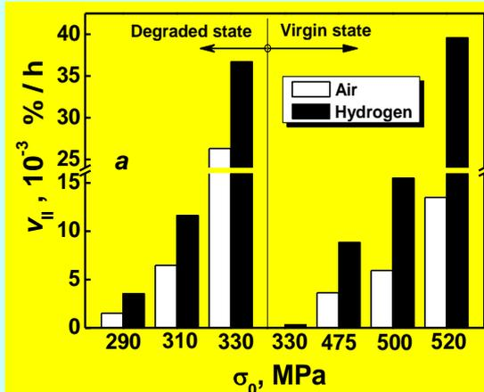
The steady-state creep rate  $v_{II}$  at different initial stress levels  $\sigma_0$  during creep test at a temperature of 450 °C for the 2.25Cr-Mo steel in virgin state (on the right) and after  $\sim 6 \cdot 10^4$  h holding inside oil hydrocracking reactor as a "specimen-witness" (on the left) obtained in air (white) and hydrogen (black bars).
