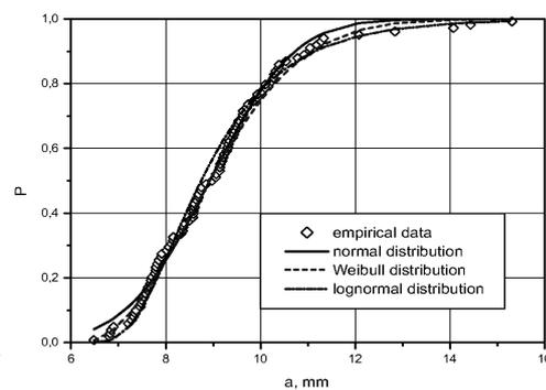
Fig. 2. C. d. f. of final crack length
