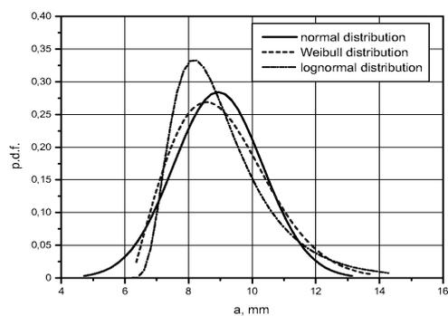
Fig. 1. P. d. f. of final crack length
