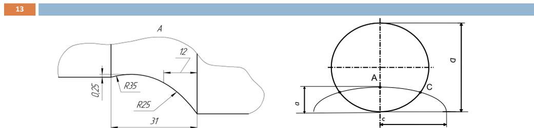
Fig. 1. Dimensions of axle fillet
