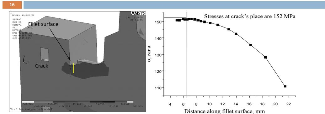
Fig. 1. Stress distribution on the surface of fillet.
