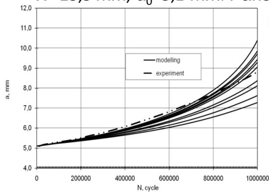
Fig. 1. Crack length  $a$  vs.  $N$ ,  $a_0 = 5,1$  mm
