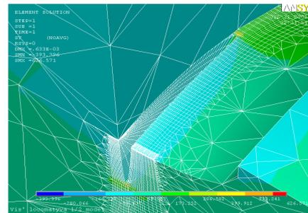
Fig. 1. Stress distribution and detail of the mesh for a crack with  $a = 16.0$  mm and  $a/c = 0.4$ .
